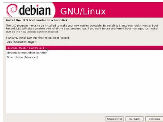
Gambar 2.53 Lilo Installation target
